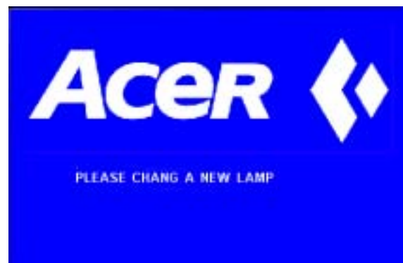
Figure 19 Lamp replacement warning signal III
