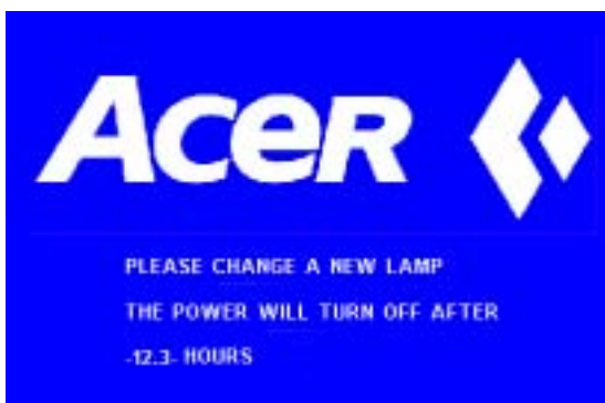
Figure 18 Lamp replacement warning signal II
