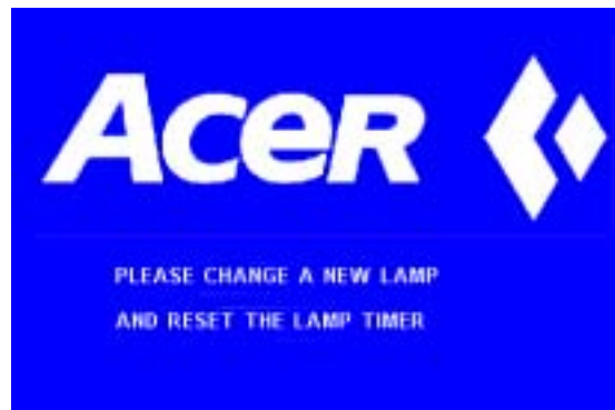
Figure 17 Lamp replacement warning signal I
